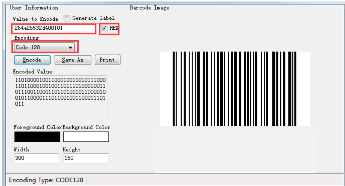
1) Check the “HEX” and send the setup code data to the data frame (no spaces in the middle).
